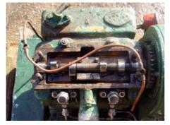
attach the sprocket to the starter shaft using slotted holes (access through rear access panel) and adjusting its relative position, then retightening the nuts. The TDC position of the piston, indicated by the relative cylinder mark (1 or 2) aligned with the PMS datum on the flywheel housing should coincide with the camshaft lobes "rocking" between the inlet closed and exhaust open position for either cylinder 1 or 2 as appropriate.
