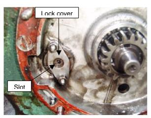
By slackening off the two nuts on the lock cover the pivot shaft for the cam levers can be rotated. The mounting of the shaft is eccentric, and therefore by rotating the shaft the axis of the cam lever pivot can be raised or lowered.
