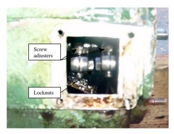
The cam levers act on each of the two individual injection pistons in the injector pump. Adjust the clearance on the pump followers by slackening off the lock nuts and screwing the adjuster up or down. When adjustments are complete retighten the lock nuts.
