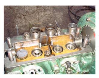
The tappets are inverted cups with 4 small lubricating holes. They are machine fitted in the cylinder head recess for the double valve springs. On the top of the valve stem is fitted a small machined cap. This cap sits above the valve spring retaining collets. It is by the replacement of this cap with others of various thicknesses that the required valve clearances are achieved.
