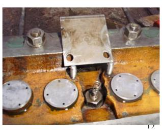
locknuts are adjust by allowing the plate to rest horizontally on the tappets of the fully closed inlet valves and locked down just touching the plate in this position.
